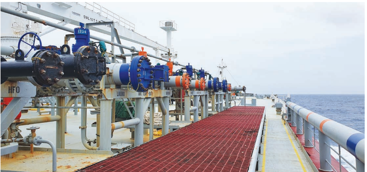
Fig 3: Gas tanker manifold – note central vapour manifolds surrounded by liquid manifolds
