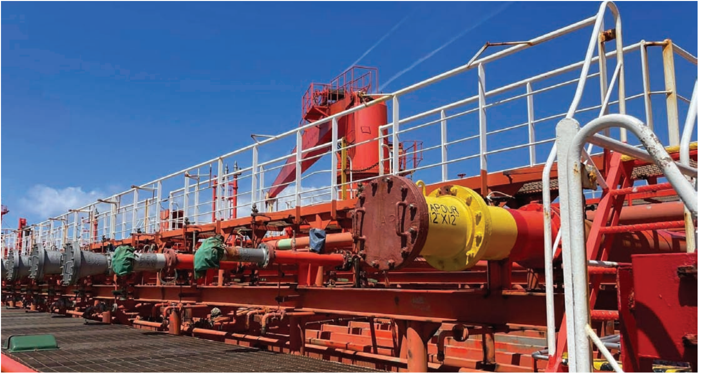
Fig 2: Oil tanker manifold – note vapour line at outer end
